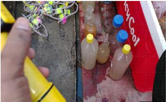
Fig. 7. On-site sample collection for DO fixation at Saryu River site, Gonda District
