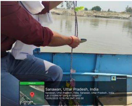
Fig. 8. On-site water sample analysis instruments: (a) Secchi disc depth measurement, (b) pH measurement at Saryu River site, Gonda District
