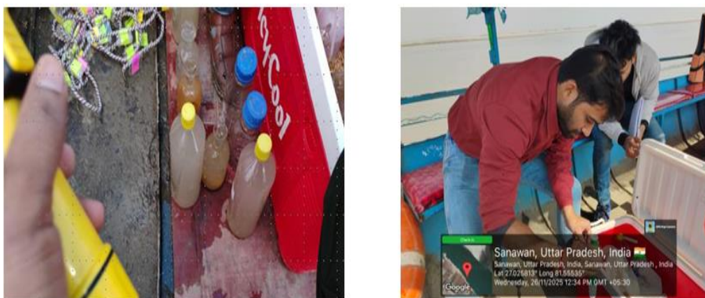
Fig. 5. On-site sample collection for DO fixation at Ghaghara River site Barabanki
