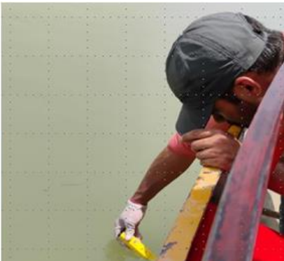
Fig. 8. On-site water sample analysis instruments: (a) Secchi disc depth measurement, (b) pH measurement at Saryu River site, Gonda District
